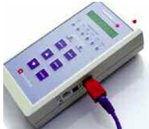
ParticleScan with crossover adapter and network cable for direct connection to the ethernet port of a computer.
