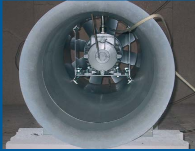
Certification test of axial fan HA, (above) and centrifugal roof fan DVV
