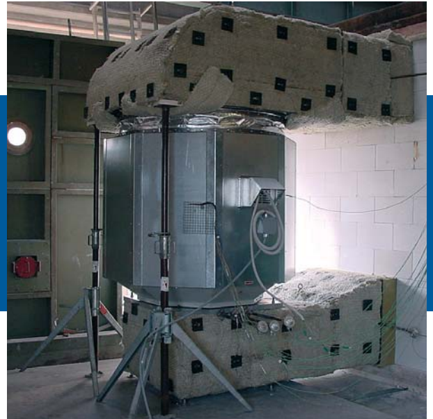
Certification test of axial fan HA, (above) and centrifugal roof fan DVV
